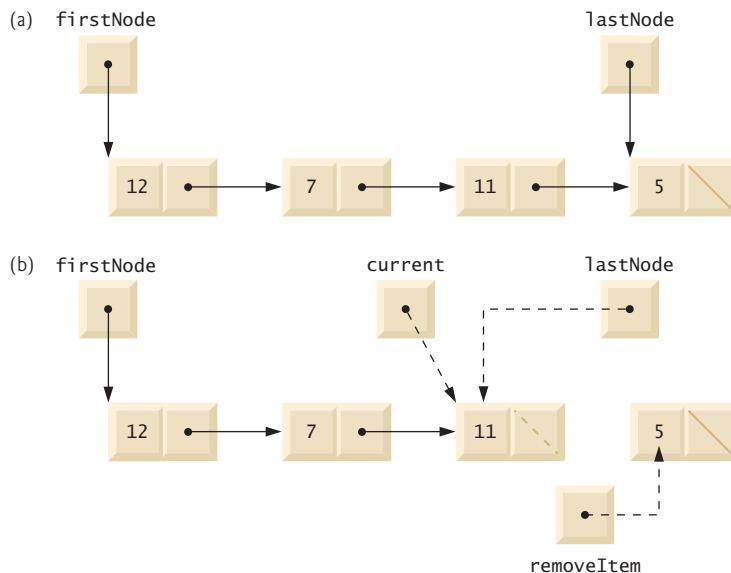
**Fig. 21.9** | Graphical representation of operation `removeFromBack`.
