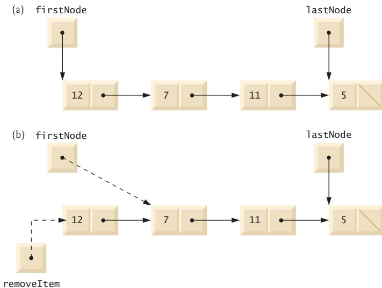
**Fig. 21.8** | Graphical representation of operation `removeFromFront`.
