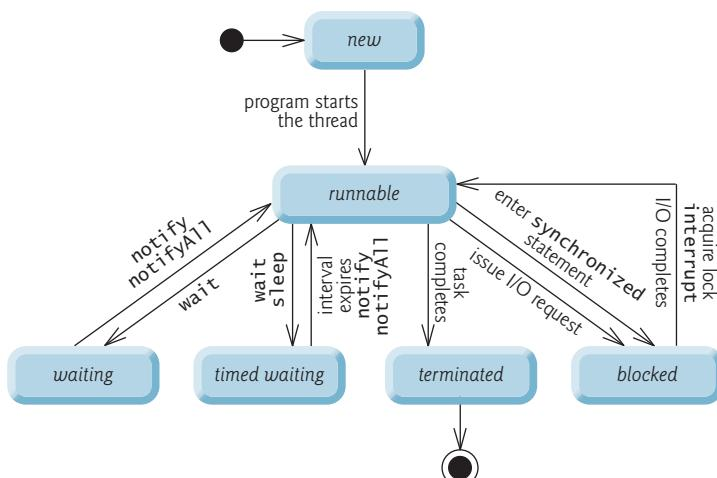
**Fig. 23.1** | Thread life-cycle UML state diagram.
