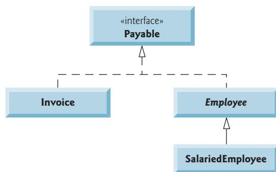
**Fig. 10.10** | Payable hierarchy UML class diagram.
